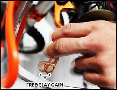
3. Adjust the install gap to achieve Free Play gain between 1/8"-1/4" (3-6mm)
