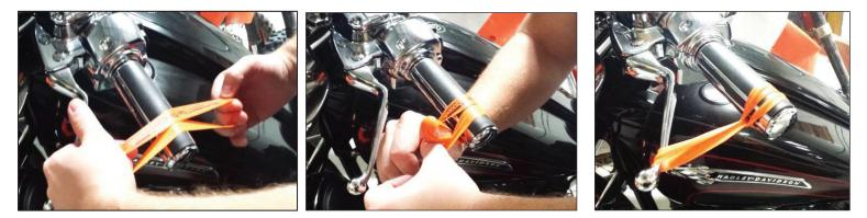
e) While still in **NEUTRAL**, quickly rev the engine between 3,000-5,000 RPM (1/4 to 1/2 throttle), then let it return to idle. Notice the movement in the clutch lever when the engine is revved. This is your Free Play Gain.
