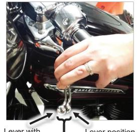
Lever with "slack" removed Lever position around 4,000 RPM
