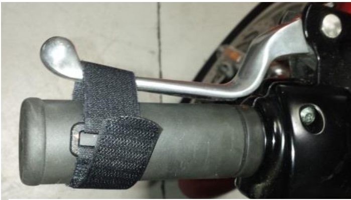
Clutch Lever Strap: to prevent unwanted launching.
