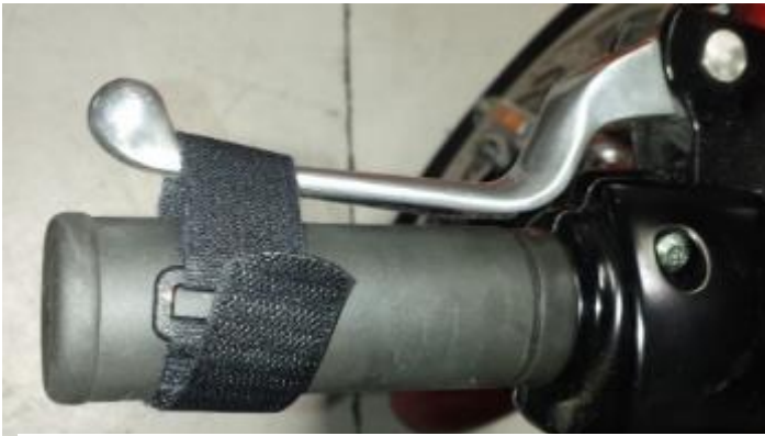
Clutch lever strap: Use to prevent unwanted launching
