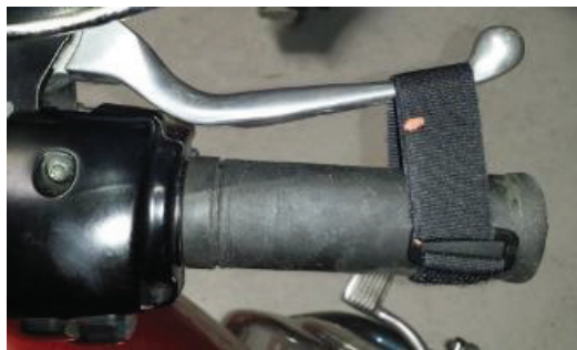
Brake lever strap: Use as a parking brake.
