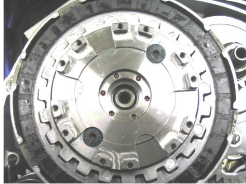
Rotate Rotating Hub and install remaining 2 - M5 screws.
