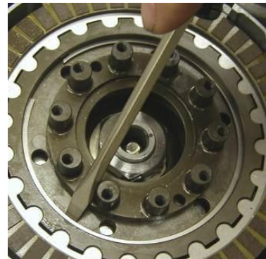
Threading retaining ring into groove
